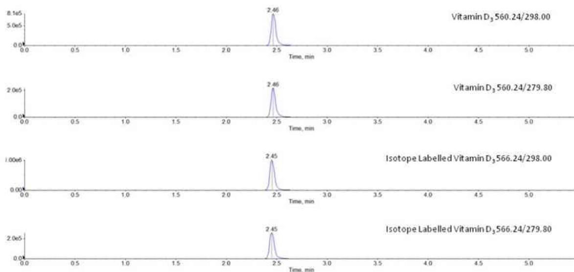
**Figure. 1** Chromatograms of quantifier and qualifier ions of PTAD-derivatized vitamin D<sub>3</sub> and PTAD-derivatized hexadeuterated vitamin D<sub>3</sub>.
