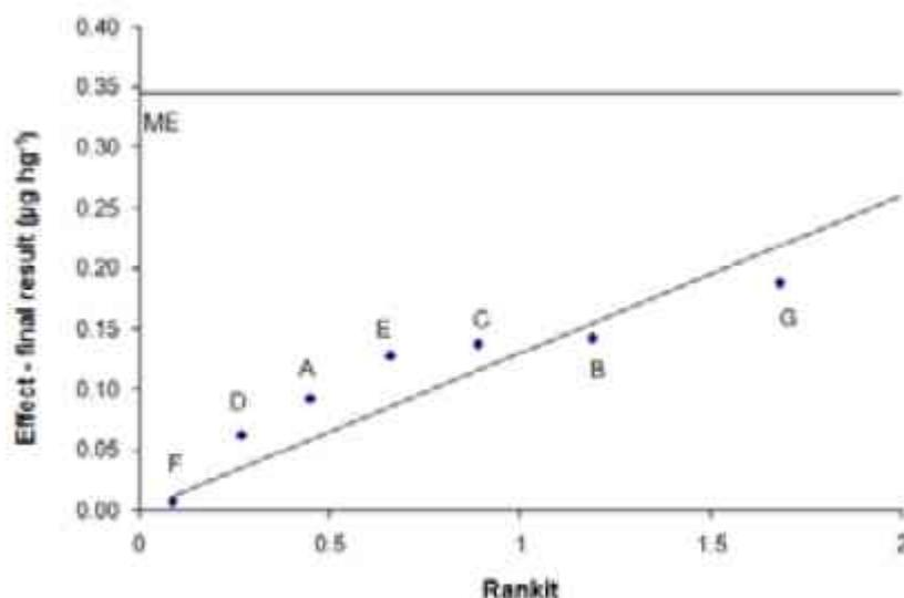
**Figure. 3** Half-normal plot of robustness results: A = water bath temperature; B = saponification time; C = isooctane volume; D = horizontal shaker time; E = isooctane transfer volume; F = PTAD volume; G = derivatization time; and ME = margin of error.
