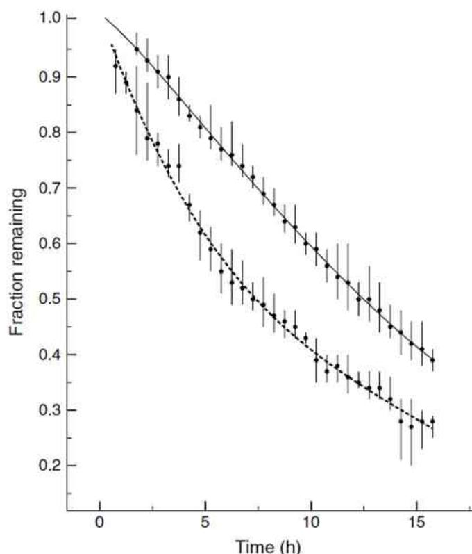
**Figure. 3** Fraction of primary amine groups remaining during the course of curing of UF resin alone (solid line) and UF resin with 3% wood fiber added (dashed line). Error bars show the range of values obtained for five replicates.
