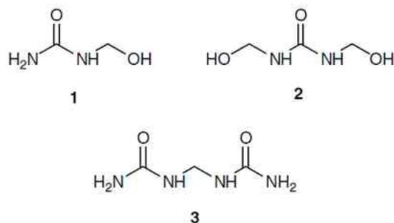
Natural abundance  $^{15}\text{N}$  NMR has been used to study UF resins<sup>1</sup> and it was found that it was possible to distinguish nitrogens in differing chemical environments within the resin; changes were observed upon curing with reduction of peaks associated with low molecular weight moieties such as **1** and **2** and of the peak for urea. In this study, 20000 scans were used to acquire spectra.
